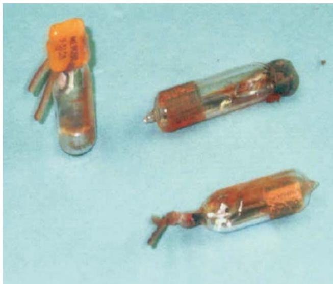
Fig.3. Switches can contain a teaspoon or more of liquid mercury.
